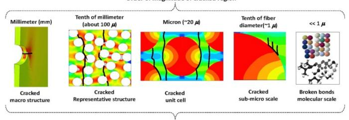
Damage at different length scales
